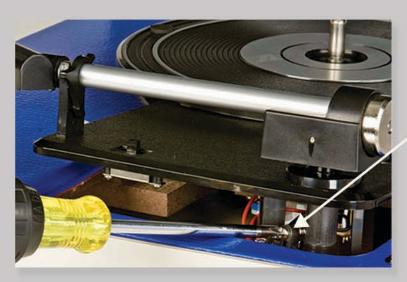
Step 3: Using a Phillips head screw driver, turn the chrome screw COUNTER-CLOCKWISE in half turn increments to extend the playing time.
